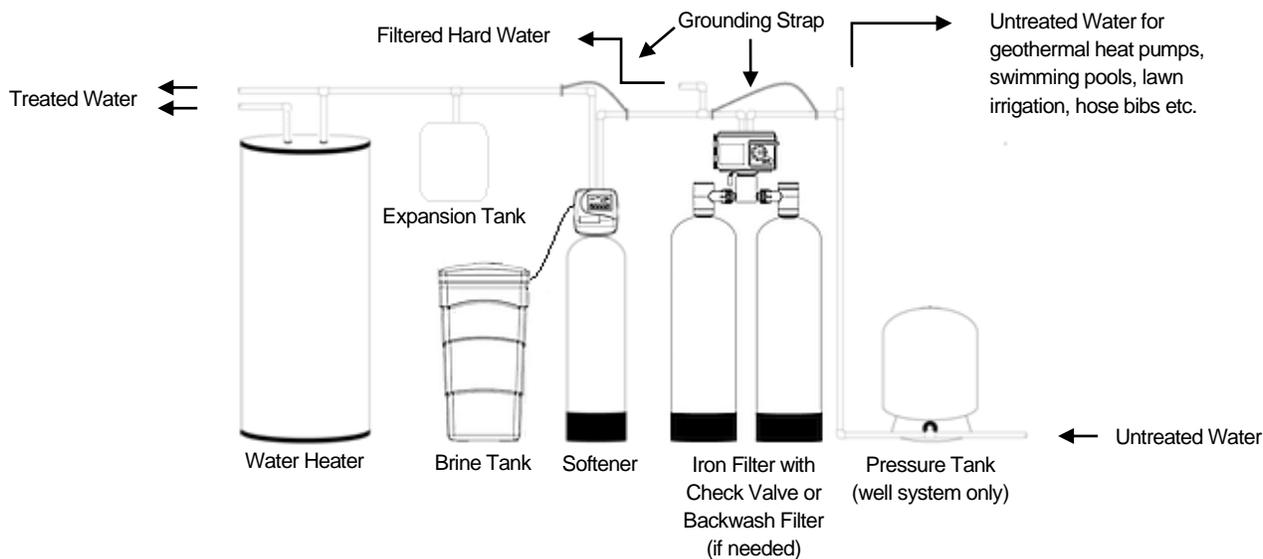
FIGURE 1: Typical Installation
